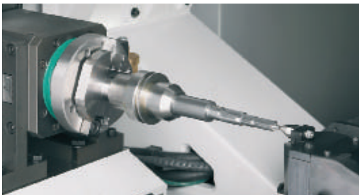
Machining between centres
