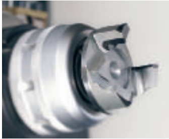
Tool with internal cutting edges (bell-shaped tool)
