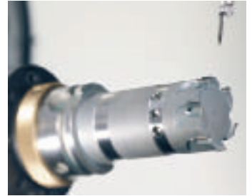
Circular milling tool
