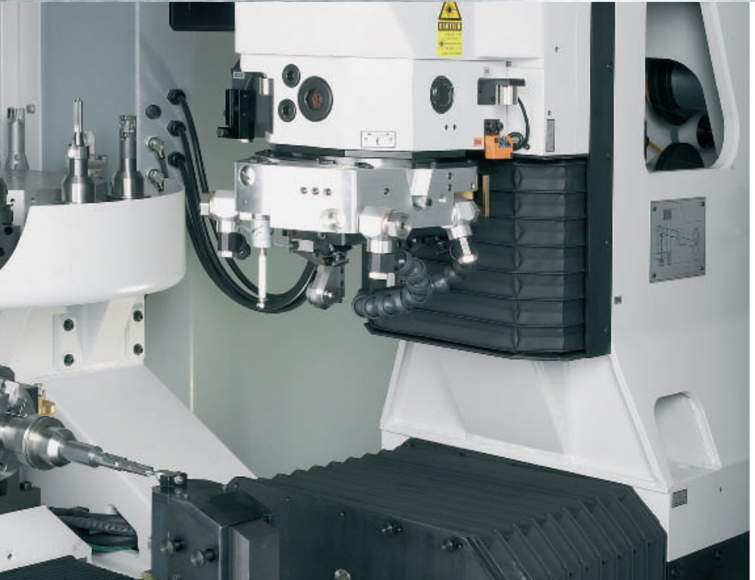
QWD 760 H with magazine for metal cutting tools: clamps shank-type tools from 85 to 390 mm in length, with a machining length of 350 mm
