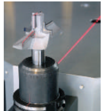
Alignment of tool in magazine
